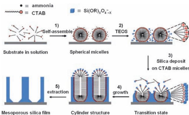
Figure 4. Illustration of the formation process of ordered mesoporous silica films with perpendicular mesochannels by the Stöber-solution spontaneous growth procedure.
